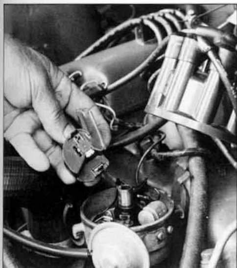
John H. holds the rev limiter. Housed in the twin point-dizzy, it may be small but does a good job, cutting in without fail at 6200 rpm.
